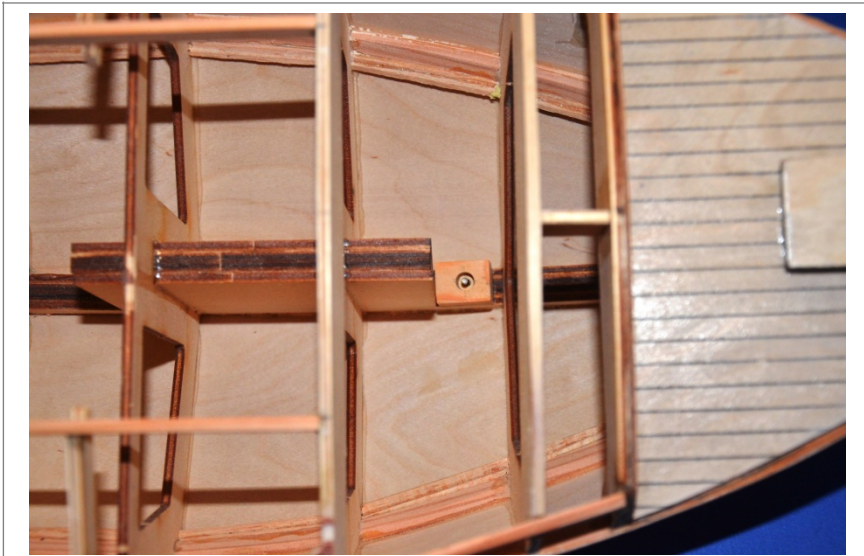
Photo 14. Mast Footing Bonded into Position
