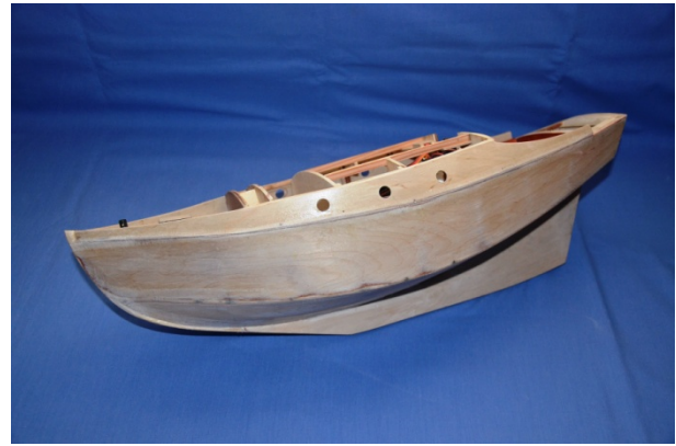
Photo 22. Cabin Sides Fitted
