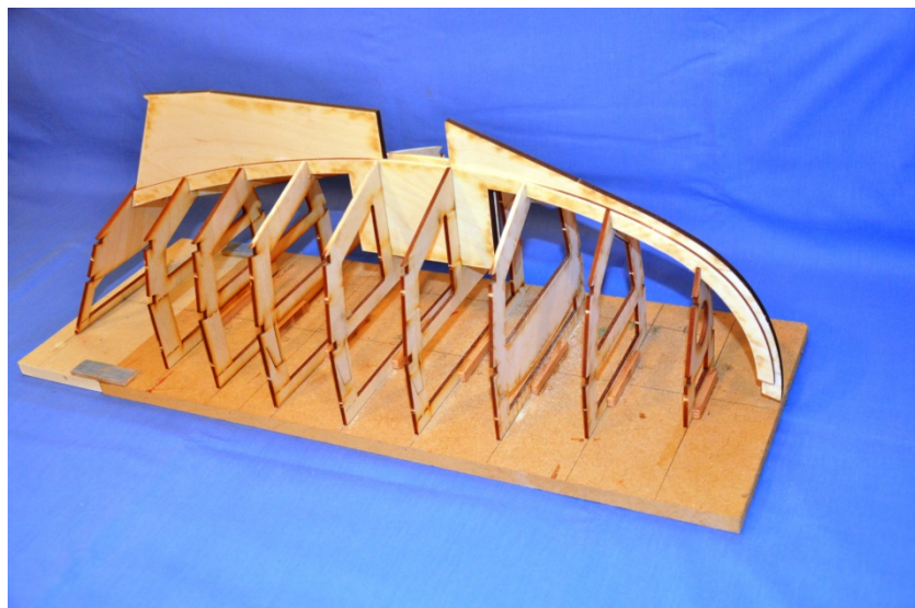
Photo 05. Bulkheads and Keel Bonded into Position
