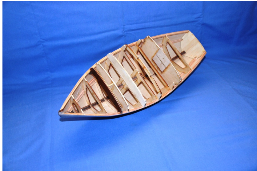
Photo 11. Hull Removed from Base Board and additional Bulkheads Fitted
