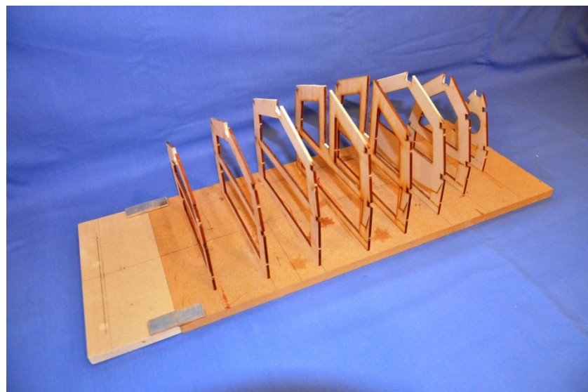
Photo 04. Bulkheads Spot Bonded to Assembly Jig
