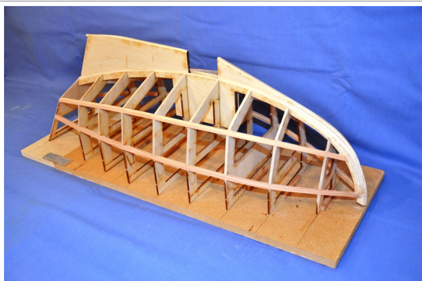
Photo 07. Second Layer of Stringers Fitted
