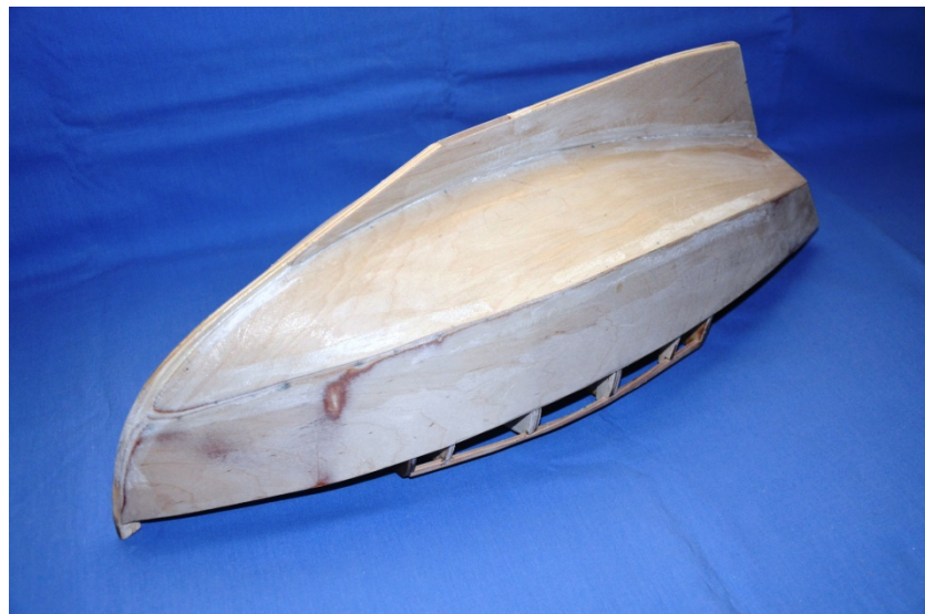
Photo 20. Hull Final Covering & Sanded
