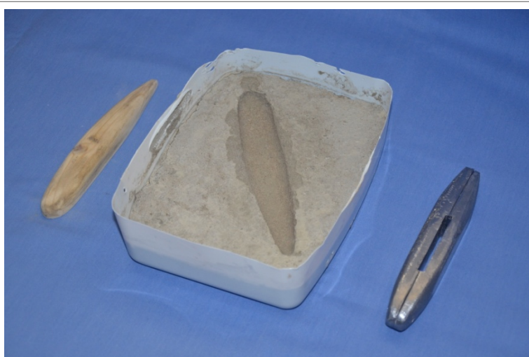
Photo 29 Male Plug, Female Mould and Cast Ballast Weights
