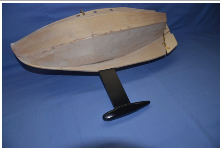
Photo 31 Painted and Fitted Keel
