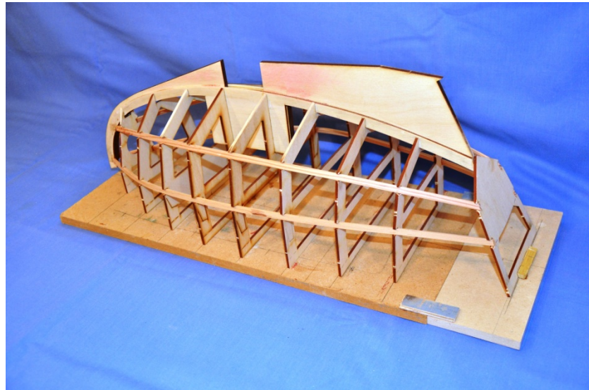
Photo 06. First Layer of Stringers Fitted
