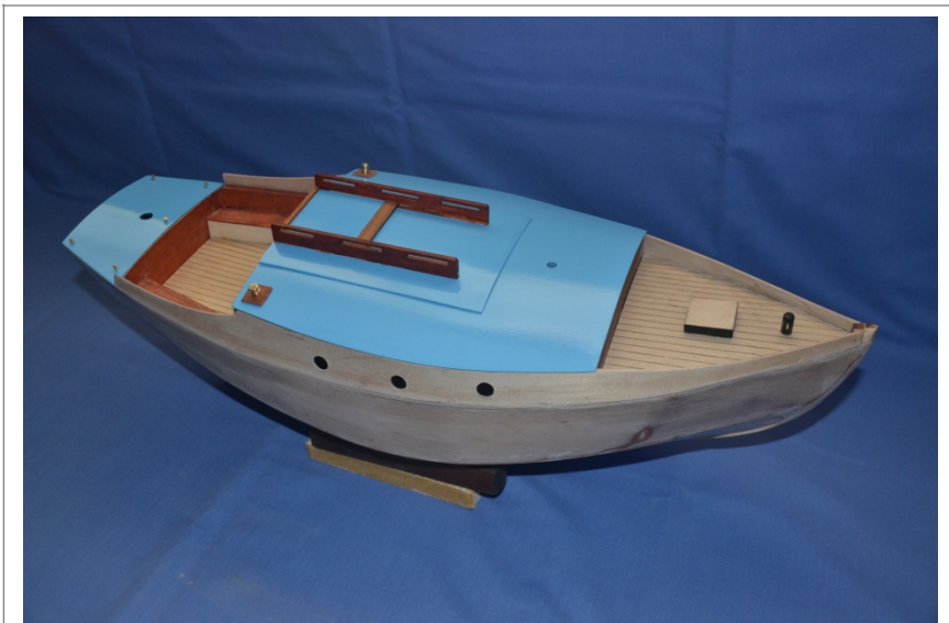
Photo 24. Cabin Roofs Temporary Fitting
