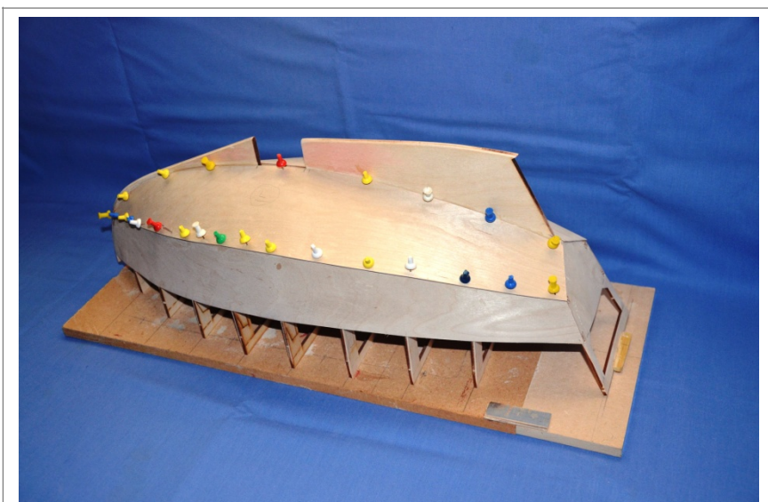
Photo 09. Hull Bottom Pinned and Glued into position
